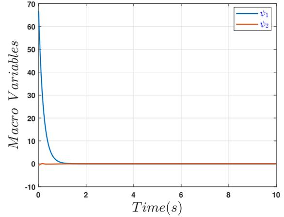
Fig. 9. The synergetic macro variables of the proposed controller.
