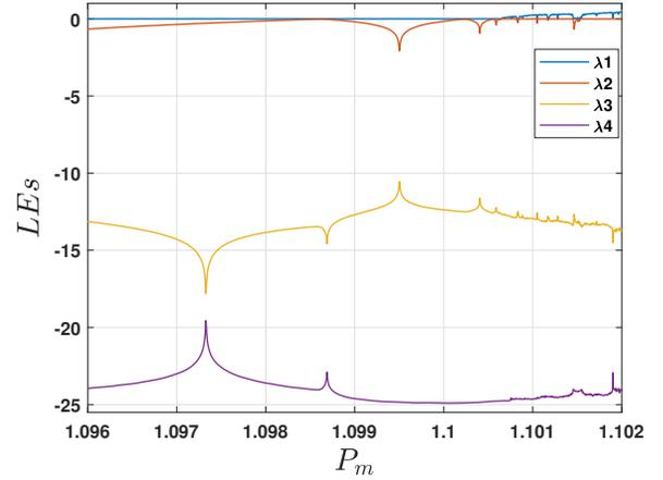
Fig. 4. Lyapunov spectrum for the power system (1) varying with  $P_m$ .
