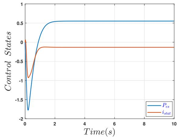
Fig. 11. Active power absorbed by the energy storage device and the STATCOM compensator current.
