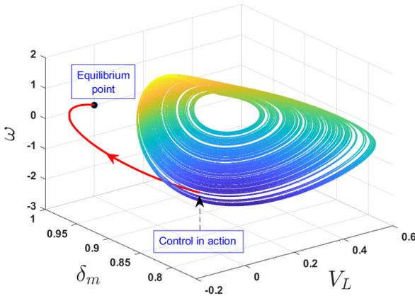
Fig. 13. Phase diagram of the controlled power system (3) with control in action at  $t = 175$  (s). The red line represents the trajectory leaving the chaotic attractor.
