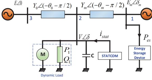
Fig. 2. The complete controlled power system (3) circuit diagram.
