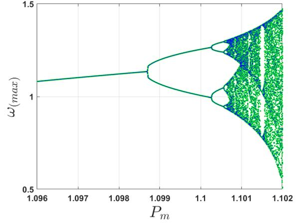
Fig. 3. Bifurcation diagram of the chaotic power system (1) for the system state  $\omega$  varying with  $P_m$ .
