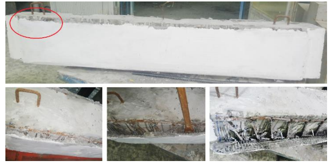
Fig. 14 The (S.-J. + Ferrocement + R) beam after the failure.
