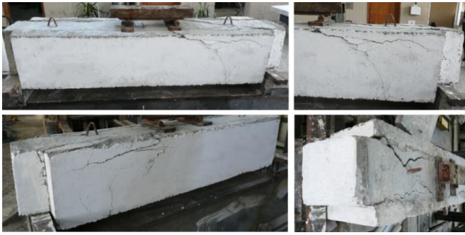
Fig. 12 The (S.-J. + Stirrup) beam after the Testing.
