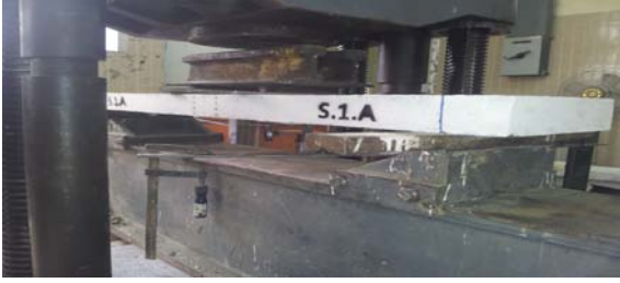
Fig. (5): Picture of the slab in the testing machine.
