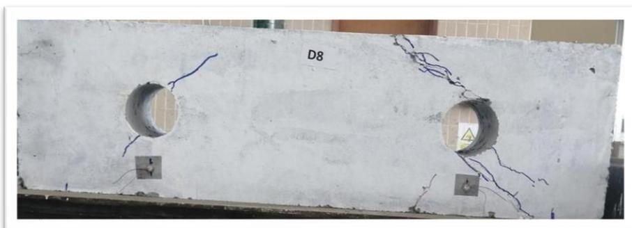
Figure 11. Shear cracks pattern of D8
