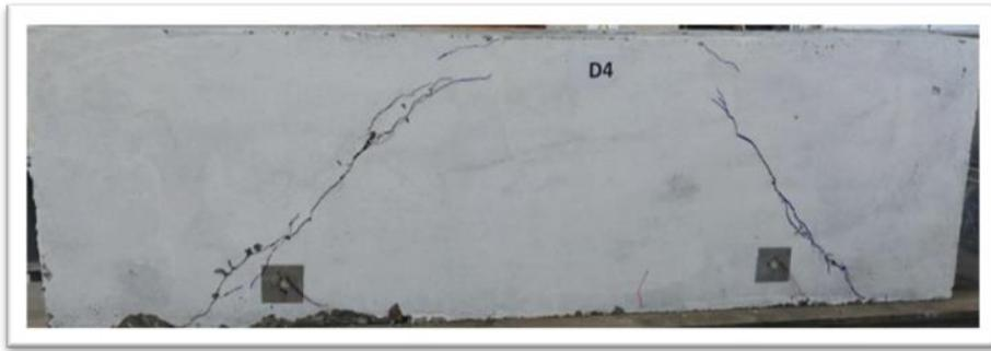
Figure 7. Shear cracks pattern of D4
