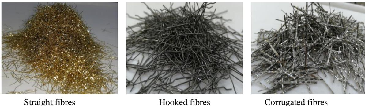
Figure 2. Type of steel fibres
