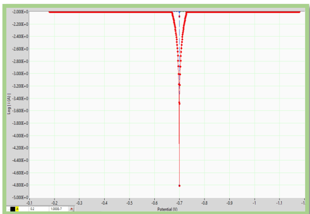
Fig. 7. Tafel curve for C-steel at 323 K in 1 M HCl (blank).
