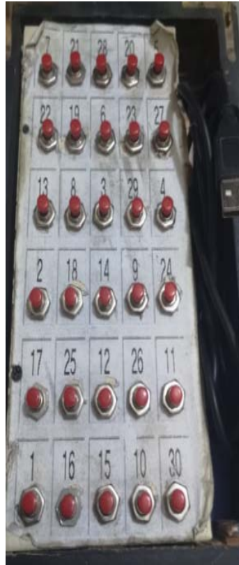
Figure 1. Shows the keyboard box to test the accuracy of the compatibility between hands and eyes
