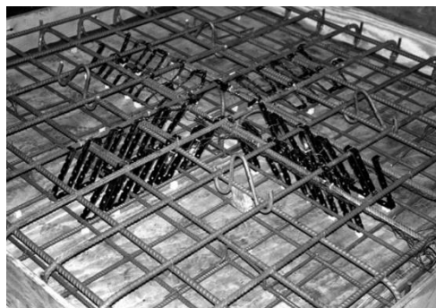
Figure (13): Reinforcement in slab Punching Shear Slab [15]
