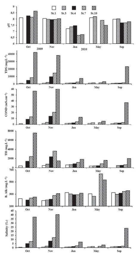
Fig. 2. Changes in physical and chemical characteristics at stations along the Shatt Al-Arab. (TDS, total dissolved solids; COND, conductivity; TH, total hardness; B.Alk, bicarbonate alkalinity).
