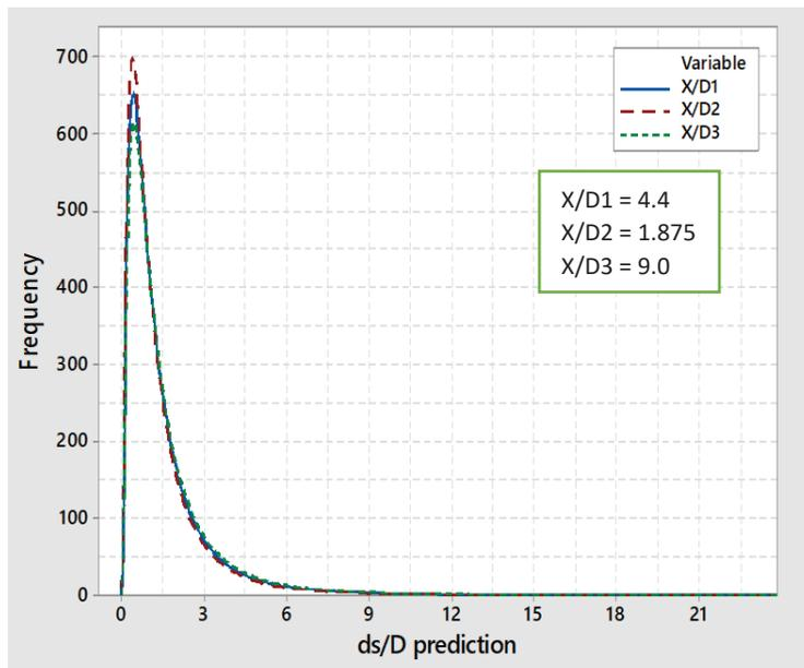
**Figure 8:** Lognormal distribution of local scour over pier diameter
