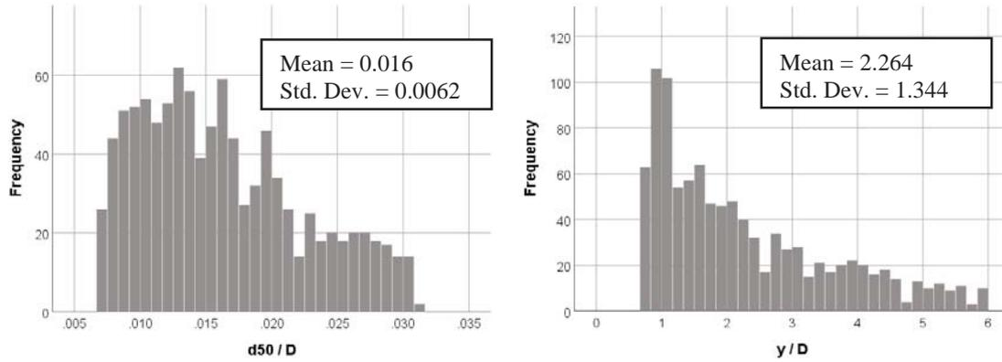
**Figure 7:** Distribution types of parameters in the equation of local scour (N=1000)
