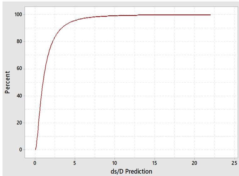
**Figure 9:** Cumulative probability distribution of local scour values over pier diameter
