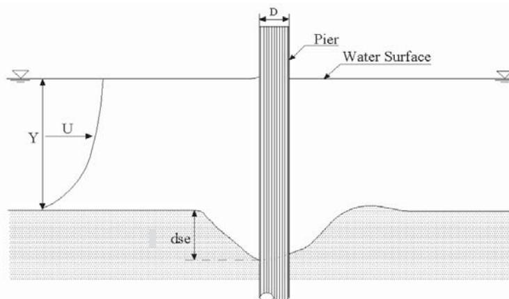
**Figure 1:** Section profile of scouring around the circular pier [12]
