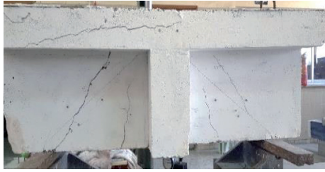
FIGURE 36: Strain and crack patterns at failure load for GTB.
