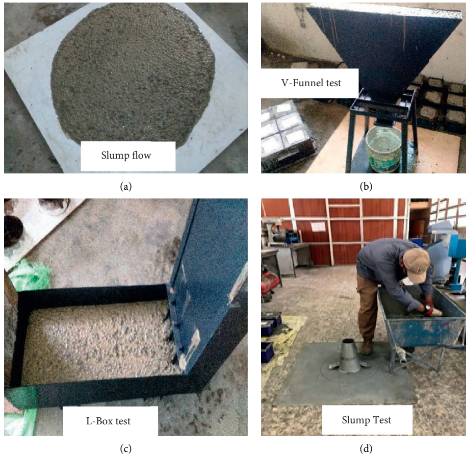
FIGURE 5: L-box, v-funnel, slump flow, and T50 tests.
