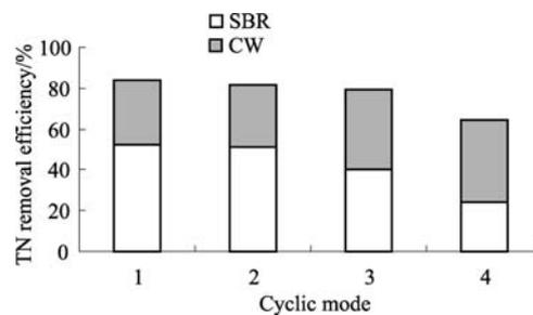
Fig. 8 Total nitrogen (TN) removal efficiency by combine process of different cyclic modes 1 to 4
