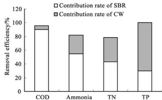
Fig. 10 Removal efficiency of chemical oxygen demand (COD), ammonia, total nitrogen (TN), and total phosphorous (TP) in combined process
