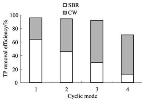
Fig. 9 Total phosphorous (TP) removal efficiency by combining process of different cyclic modes 1 to 4
