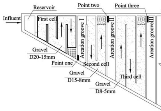
Fig. 3 Constructed wetland plan view
