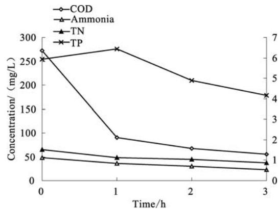
Fig. 11 Relationship of COD (chemical oxygen demand), ammonia, TN (total nitrogen), TP (total phosphorus) in the 3rd cycle of sequencing batch reactor
