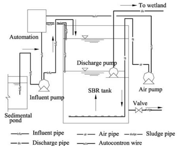
Fig. 2 Sequencing batch reactor (SBR) system
