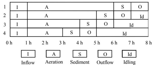
Fig. 4 Sequencing batch reactor operate cycle
