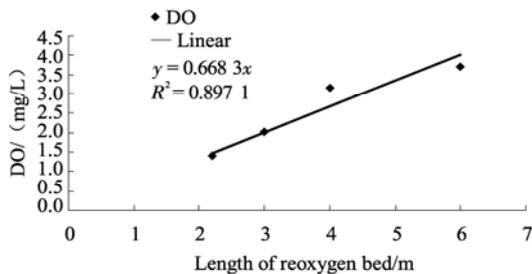
Fig. 7 Relationship between dissolved oxygen (DO) and length of reoxygenation bed
