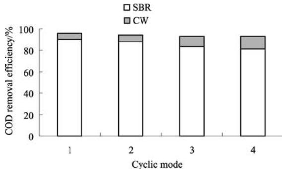
Fig. 5 Chemical oxygen demand (COD) removal efficiency by combination process of different cyclic modes 1 to 4
