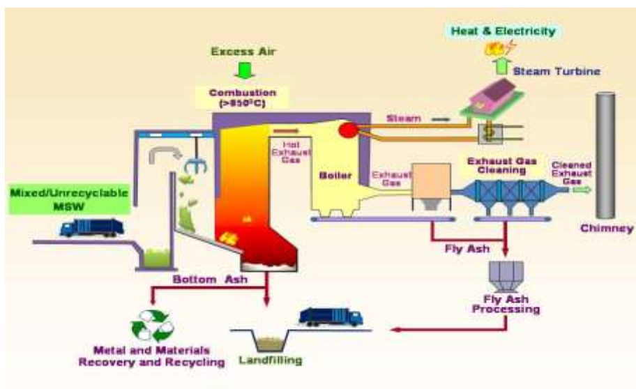
Fig. 1: The typical processes in an WTE plant
