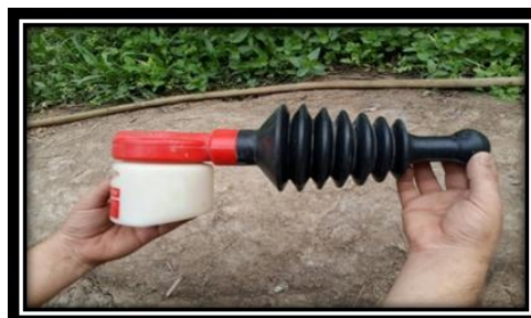
Figure 4. A fogger device that used to dust the P. harmala seed powder.
