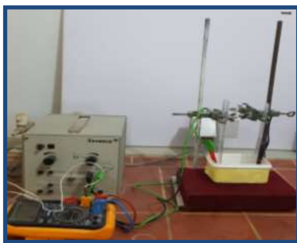
Figure 1: Anodisation unit used for preparing of TiO 2 nanotubes.
