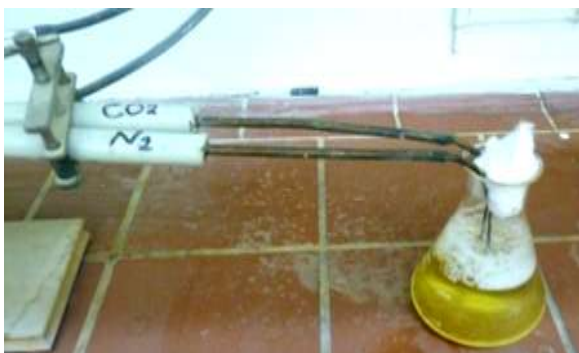
( Figure 1) Saturated media with \text{N}_2 and \text{CO}_2
