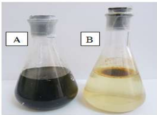
( Figure 4 ) A: Degradation of crude oil by SRB
