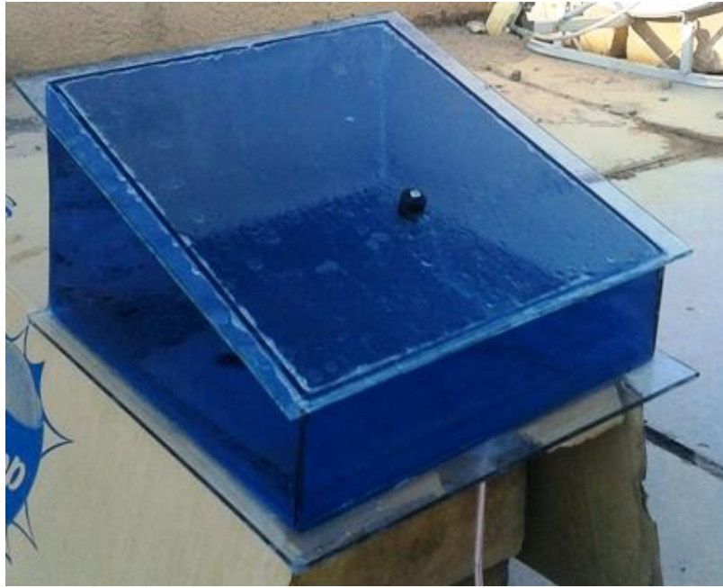
Figure 2: A photographic picture of the Single Slope Solar Still (glass one face reflector)
