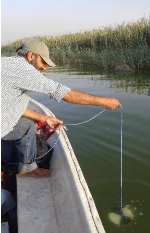
Measuring light penetration to calculate water transparency at the Manthori research station
