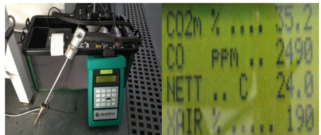
Fig. 5. Quintox devices are used to make a gas measurement.
