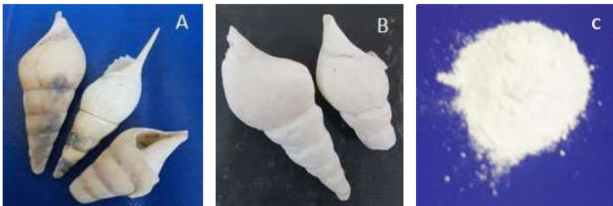
FIGURE. 1. Image for the oysters: A: prior to scraping the shell; B: after scraping the shell; C: after milling (powder).
