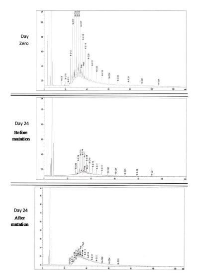
**Figure 3.** Capillary gas chromatography results of n-alkanes of bacterial mixture at day zero, day 24 before mutation and day 24 after mutation.
