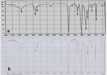
**Figure 3** IR absorption spectrum of extracted and standard reuterin. a. Standard reuterin, b. extracted reuterin produced from local isolates.
