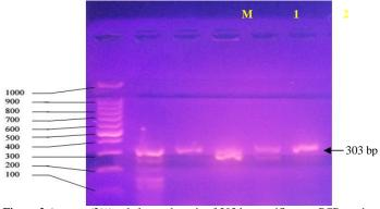
**Figure 2** Agarose (2%) gel electrophoresis of 303 bp specific gene PCR products for *L. reuteri* isolates under UV transilluminator. Lane (M): 1Kb (100 bp - 1000 bp) DNA ladder. Lane 1: isolate 1 . Lane 2: isolate 2 . Lane 3: isolate 3 . Lane 4: isolate 4 . Lane 5: isolate 5 .
