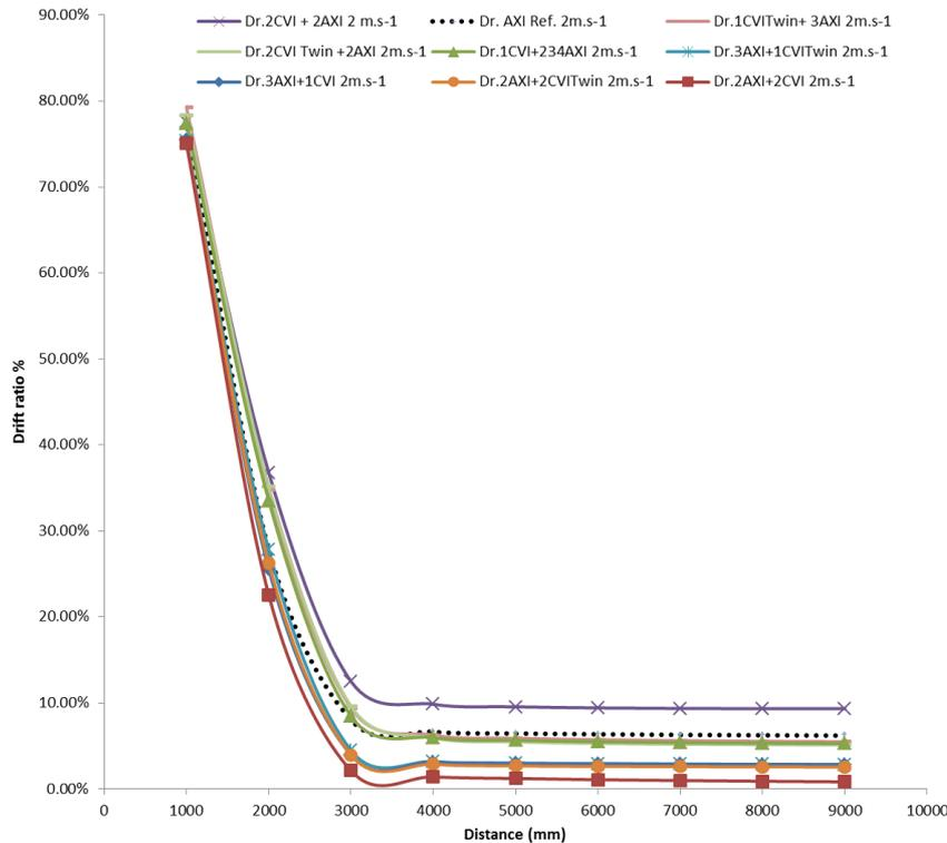
Figure 11 Effect of nozzle substitution on drift ratio at 2 m s<sup>-1</sup> wind speed compared to reference nozzle
