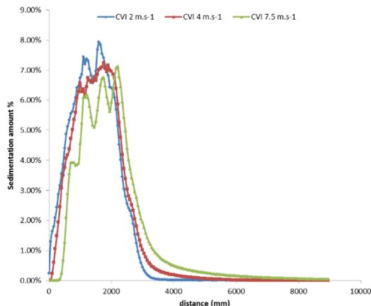
Figure 6 Deposition amount at different wind speeds using Flat Fan nozzle air induction single jet (CVI)
