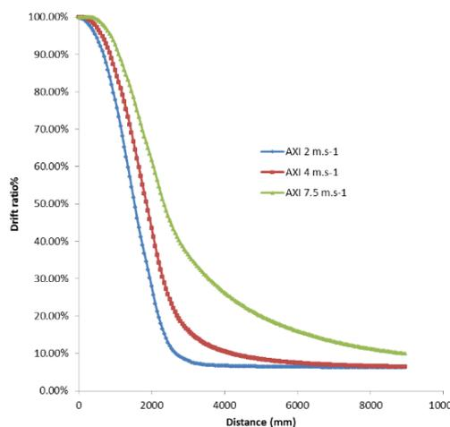
Figure 8 Effect of nozzle type on drift ratio- Flat fan nozzle (AXI)
