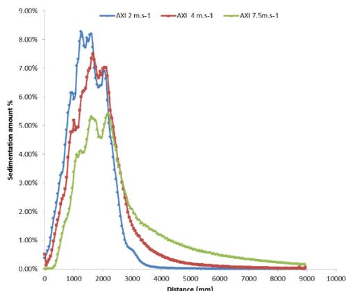
Figure 5 Deposition amount at different wind velocities using Flat Fan nozzle (AXI)
