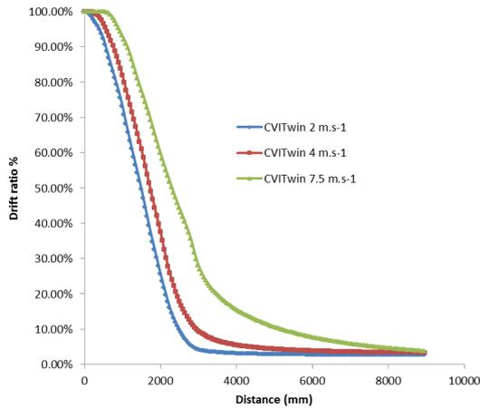
Figure 10 Effect of nozzle type on drift ratio- Flat Fan air induction Twin nozzle (CVITwin)
