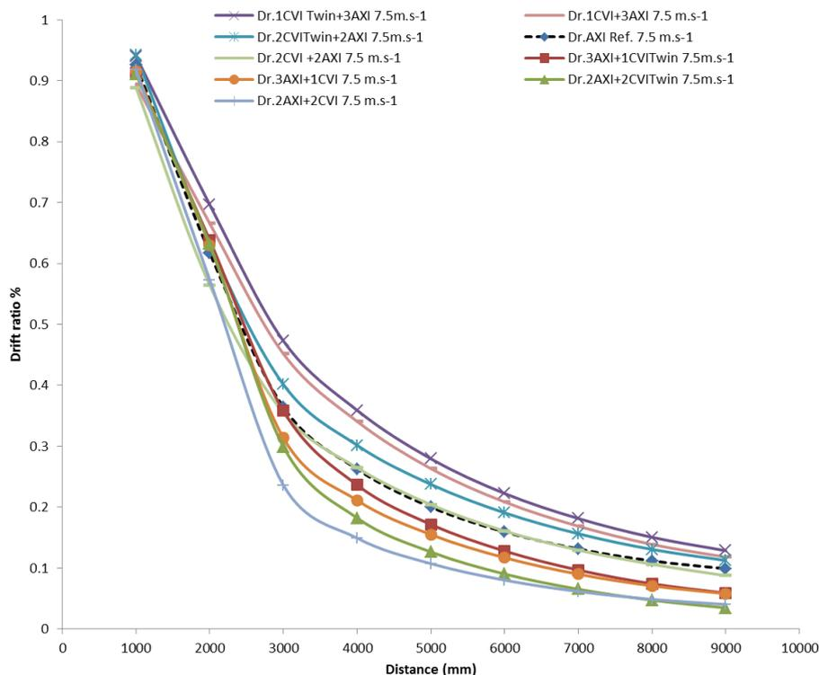
Figure 13 Effect of nozzle substitution on drift at 7.5 m s<sup>-1</sup> wind speed compared to the reference nozzle
