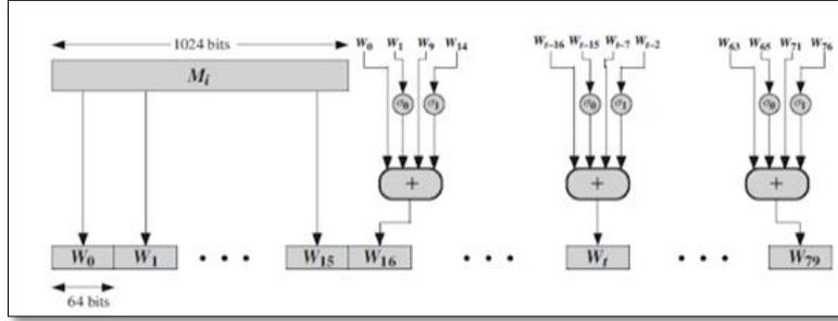
Fig. 4. Creation of 80-word input Sequence for SHA-512 processing of single block.
