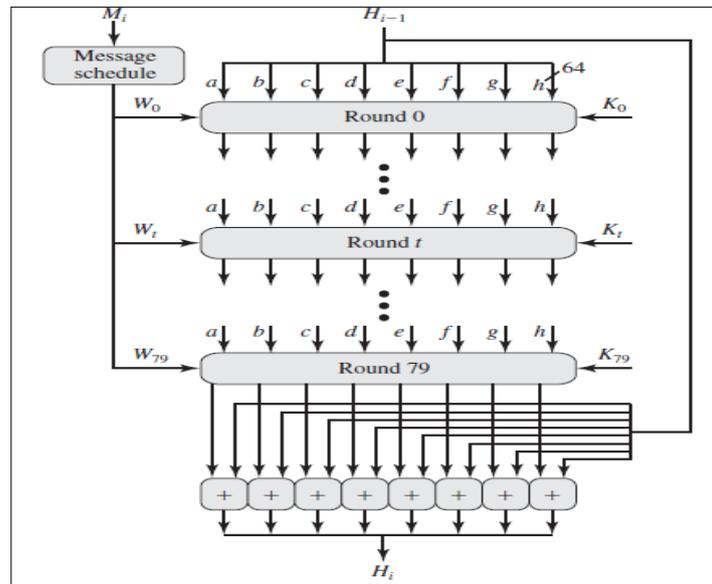
Figure 3. SHA-512 processing of a Single 1024-bit block.
