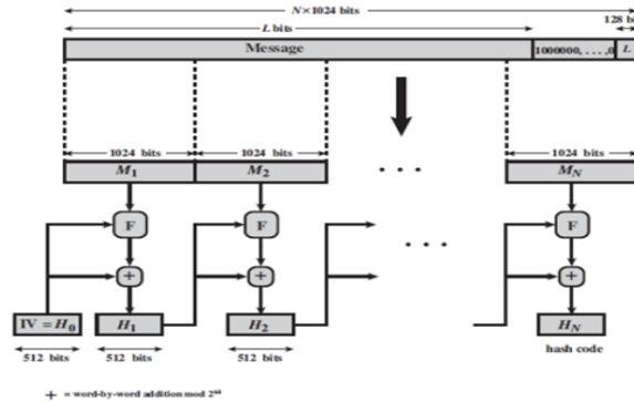
Figure 2. Message digest generation using (SHA-512).
