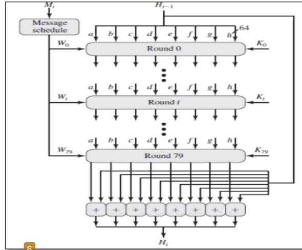
Fig. 3. SHA-512 processing of a Single 1024- bit block.
