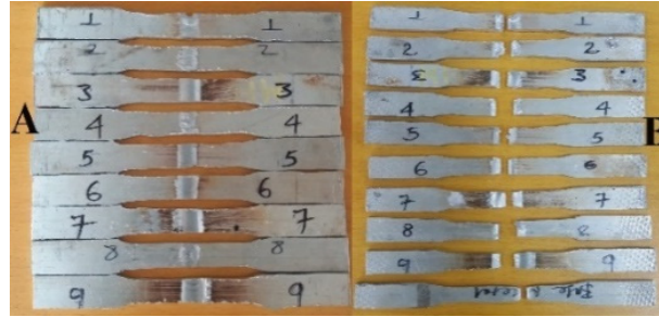
Figure 5. Extraction of tensile specimens: (A) Welded specimens before the tensile test; (B) welded specimens after the tensile test.
