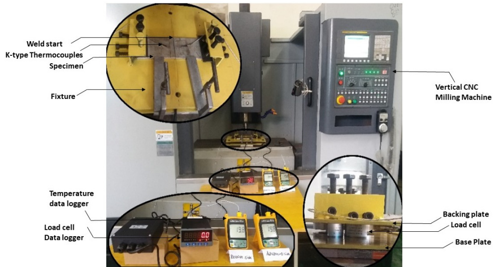
Figure 3. Experimental setup used for FSW connected with the load cell and thermocouples.
