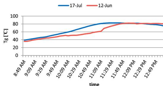
Fig. 2. Measured variation temperature of generator with Time at 12th of June & 17th of July -2019.
