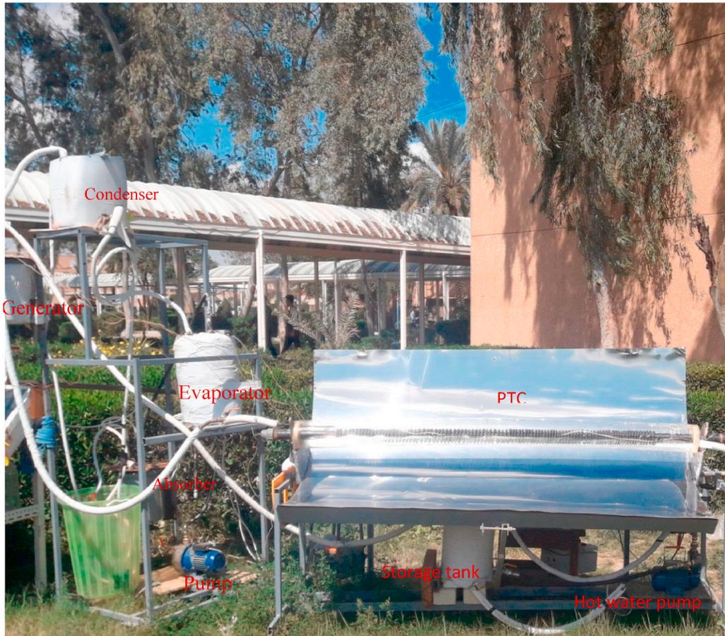
(a) The Fabricated Solar Absorption Refrigeration System
