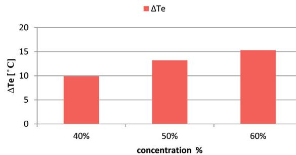
Fig. 5. Measured variation maximum temperature drop of evaporator with Variable concentration for June 2019.
