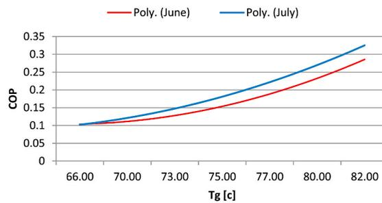
Fig. 6. Experimental COP with generator temperature of June and July 2019.
