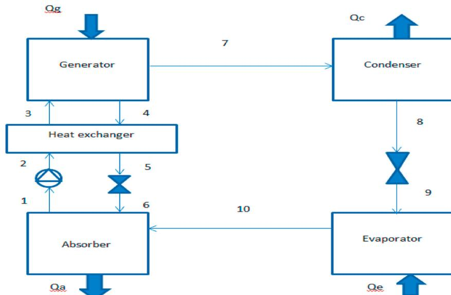
(b) Schematic of a Single cycle Absorption System
