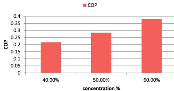
Fig. 7. Experimental maximum COP with variable concentration of June 2019.
