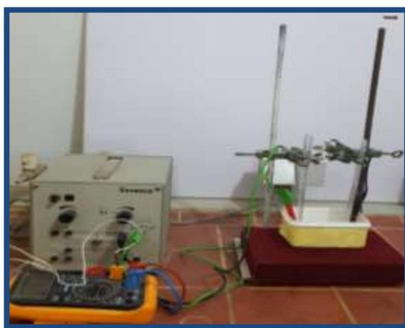
**Figure 1:** Anodisation unit used for preparing of TiO<sub>2</sub> nanotubes.
