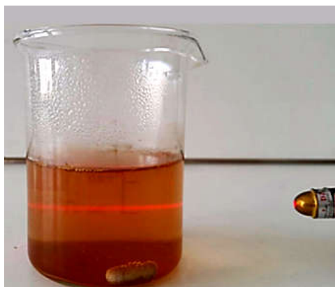
Figure 1: shows the mixture after (2) min with formation of silver nanoparticles confirmed by laser beam
