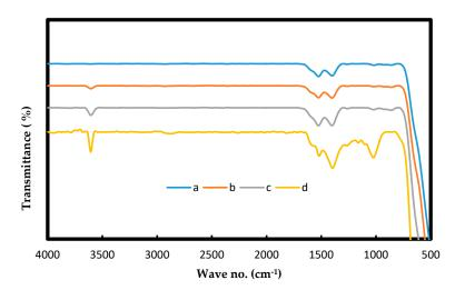
**Figure 2.** FT-IR spectra of the catalysts: (a) Pt,Pd,Ni/MgO, (b) Pd,Pd,Ni/Mg $_{0.97}$ La $^{3+}$  $_{0.03}$ O, (c) Pd,Pd,Ni/Mg $_{0.95}$ La $^{3+}$  $_{0.07}$ O, (d) Pd,Pd,Ni/Mg $_{0.85}$ La $^{3+}$  $_{0.15}$ O.
