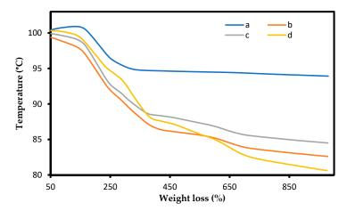
**Figure 6.** TG of the catalysts: **(a)** Pt,Pd,Ni/MgO, **(b)** Pt,Pd,Ni/Mg<sub>0.97</sub>La<sup>3+</sup><sub>0.03</sub>O, **(c)** Pt,Pd,Ni/Mg<sub>0.93</sub>La<sup>3+</sup><sub>0.07</sub>O, **(d)** Pt,Pd,Ni/Mg<sub>0.85</sub>La<sup>3+</sup><sub>0.15</sub>O.
