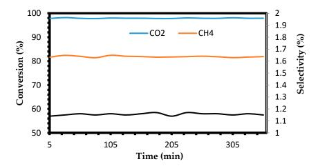
**Figure 11.** Stability tests of the Pt,Pd,Ni/Mg<sub>0.85</sub> La<sup>3+</sup><sub>0.15</sub>O catalysts at 900 °C for the 1:1 ratio of CH<sub>4</sub>:CO<sub>2</sub>, for 200 h (GHSV = 15,000 mL·g·cat<sup>-1</sup>·h<sup>-1</sup>, atmospheric pressure).
