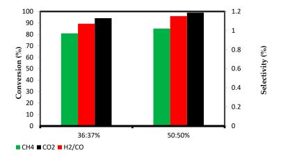
**Figure 8.** The effect of changing the ratio concentration of the  $CH_4:CO_2$  reactant a—(2:1) and b—(1:1) over the percentage of their conversion and  $H_2/CO$  ratio for Pt,Pd,Ni/Mg<sub>0.85</sub>La<sup>3+</sup><sub>0.15</sub>O catalyst at 900 °C.
