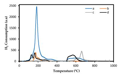
**Figure 4.** H<sub>2</sub>-TPR profiles of the catalysts (**a**) Pt,Pd,Ni/MgO, (**b**) Pd,Pd,Ni/Mg<sub>0.97</sub>La<sup>3+</sup><sub>0.03</sub>O, (**c**) Pd,Pd,Ni/Mg<sub>0.93</sub>La<sup>3+</sup><sub>0.07</sub>O, and (**d**) Pd,Pd,Ni/Mg<sub>0.85</sub>La<sup>3+</sup><sub>0.15</sub>O reduced in a (5% H<sub>2</sub>/Ar) stream at a temperature ramp of 10 °C/min.
