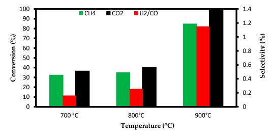
**Figure 10.** The influence of temperature on the catalytic activity of the Pd,Pd,Ni/Mg<sub>0.85</sub>La<sup>3+</sup><sub>0.15</sub>O catalyst: (1) 700 °C, (2) 800 °C, (3) 900 °C for the 1:1 ratio of CH<sub>4</sub>:CO<sub>2</sub>.
