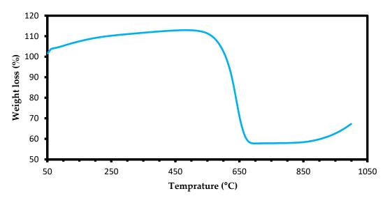
**Figure 13.** TGA profiles of the spent Pt,Pd,Ni/Mg<sub>0.85</sub>La<sup>3+</sup> $_{0.15}$ O catalyst (20 mL/min O<sub>2</sub> stream under a temperature ramp of 10 °C/min).
