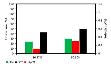
**Figure 7.** The effect of changing the ratio concentration of the  $CH_4:CO_2$  reactant a—(2:1) and b—(1:1) over the percentage of their conversion and  $H_2/CO$  ratio for the support-promoter ( $Mg_{1-x}La_xO$ ) of the catalyst at 900 °C.
