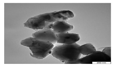
**Figure 12.** TEM analysis of the spent Pt,Pd,Ni/M $g_{0.85}La^{3+}_{0.15}O$  catalyst after reaction: at 900 °C, and CH<sub>4</sub>:CO<sub>2</sub> ratio 1:1.
