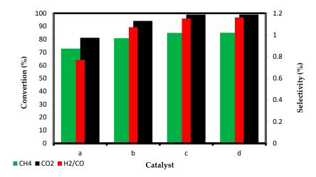
**Figure 9.** The effect of using different catalysts (a) Pt,Pd,Ni/MgO, (b) Pt,Pd,Ni/Mg $_{0.97}$ La $_{2}^{3+}$ 0.03O, (c) Pt,Pd,Ni/Mg $_{0.97}$ La $_{2}^{3+}$ 0.07O, and (d) Pt,Pd,Ni/Mg $_{0.85}$ La $_{0.15}^{3+}$ O on CH $_{4}$ , CO $_{2}$  conversion, and H $_{2}$ /CO ratio at 900 °C for the 1:1 ratio of CH $_{4}$ :CO $_{2}$ .
