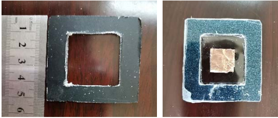
Fig. 3. The DE and the electrodes fixed on the frame at a 100% prestretch ratio.
