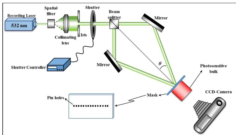
Figure 2. Schematic diagram of the setup used to monitor self-written net-waveguide.
