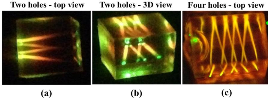
**Figure 3** Experimental observation for net-Gaussian beams evolution inside photopolymer material during SWW process: (a) and (b) two holes, (c) four holes.
