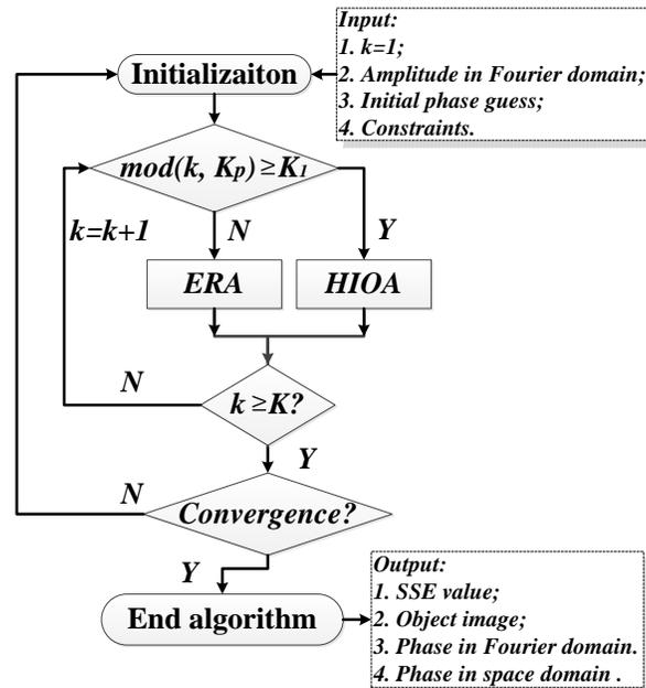
Fig. 2. Illustration of performing ER/HIO algorithm for FP reconstruction.
