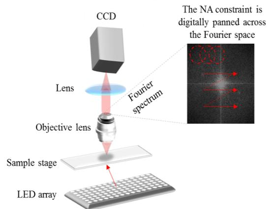
Fig. 1. Fourier Ptychographic imaging setup [2].
