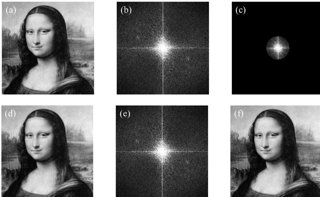
Fig. 3. Simulation results: (a) Primary high resolution intensity image, (b) Fourier spectrum of (a), (c) pupiled Fourier spectrum, (d) recovered low-resolution intensity image from (c), (e) iteratively recovered (performing ER/HIOA) full Fourier spectrum, and (f) retrieved (reconstructed) high resolution image (PSNR = 45.21 dB).
