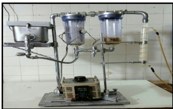
Figure 1. Ohmic distiller apparatus used for this study.
