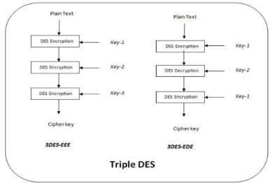
Figure1. flowchart of 3DES algorithm[9]
