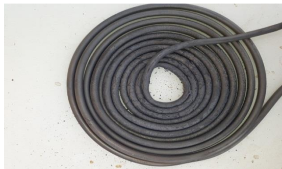
Fig. 2.b: Three meter spiral absorber
