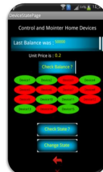
Figure (17:B) Home appliance control and monitor Screen
