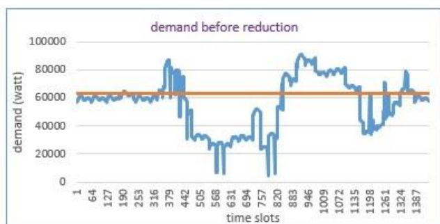
Figure 15: : total demand of ten houses, red line represent the supply threshold which covered 70% of consumer demand.
