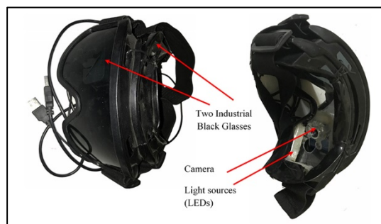
Fig. 2. Video capture system.
