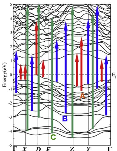
Fig. 1. The optical transitions depicted on a generic band structure of the  $\text{Ba}_2\text{Cd}_2\text{As}_3$  as prototype.
