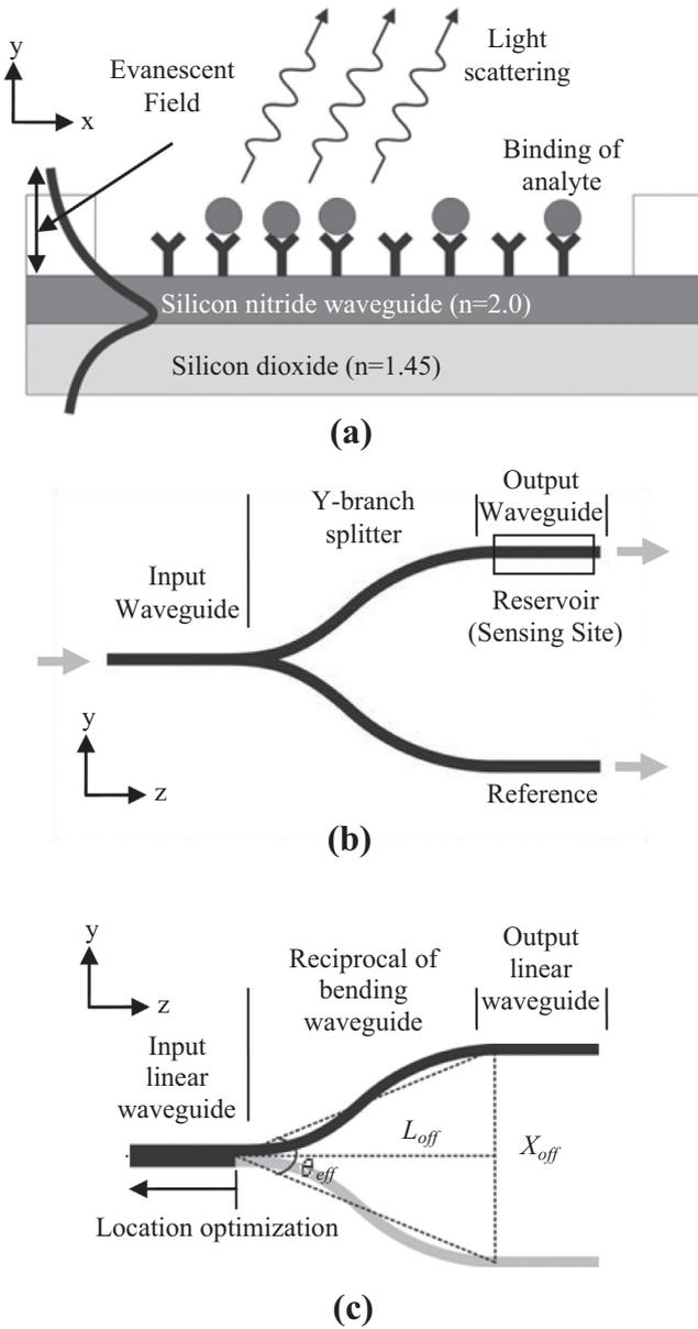
**Fig. 1.** (a) Scattering of evanescent excitation binding of analyte on the waveguide surface; (b) Y-branch splitter used as evanescent field biosensor; (c) Model of Y-branch splitter without taper.
