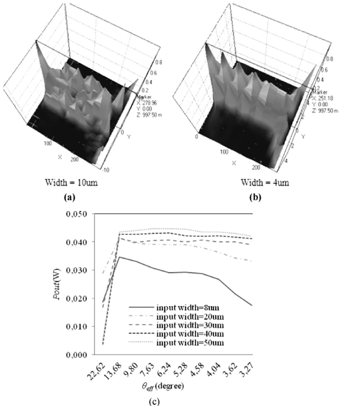
**Fig. 3.** (a) Mode beating profile of input waveguide for width of 10  $\mu\text{m}$ ; (b) 4  $\mu\text{m}$  respectively; (c)  $P_{\text{out}}$  as function of effective angle for input width of 8  $\mu\text{m}$ , 20  $\mu\text{m}$ , 30  $\mu\text{m}$ , 40  $\mu\text{m}$  and 50  $\mu\text{m}$ . Location optimization is performed only on Y-branch with input width of 8  $\mu\text{m}$  and 20  $\mu\text{m}$ .
