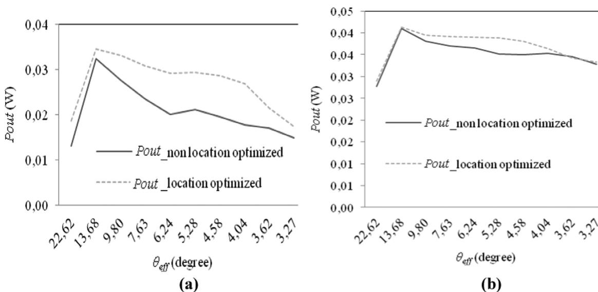
**Fig. 2.** (a)  $P_{out}$  as function of effective angle with and without location optimization for input width of 8  $\mu\text{m}$ ; (b)  $P_{out}$  as function of effective angle with and without location optimization for input width of 20  $\mu\text{m}$ .
