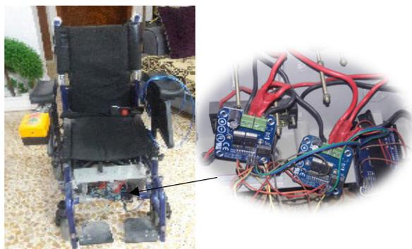
**FIGURE 21. The real picture of the wheelchair and the interfacing.**
