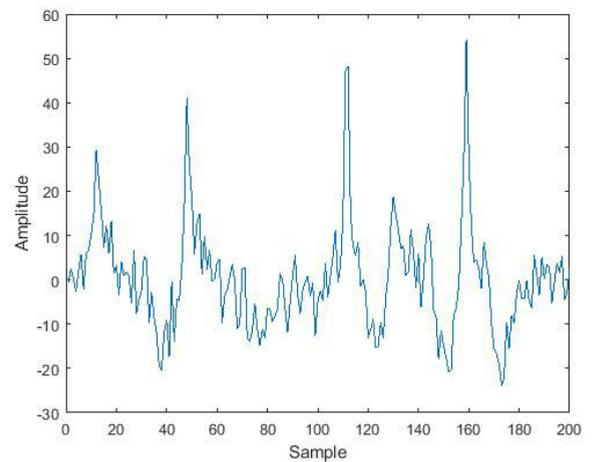
FIGURE 9. The DWT approximate coefficients of multiple eyeblinks (only ch1).
