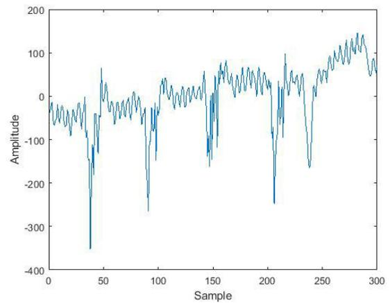
FIGURE 8. The DWT approximate coefficients of multiple jaw squeeze (only ch1).
