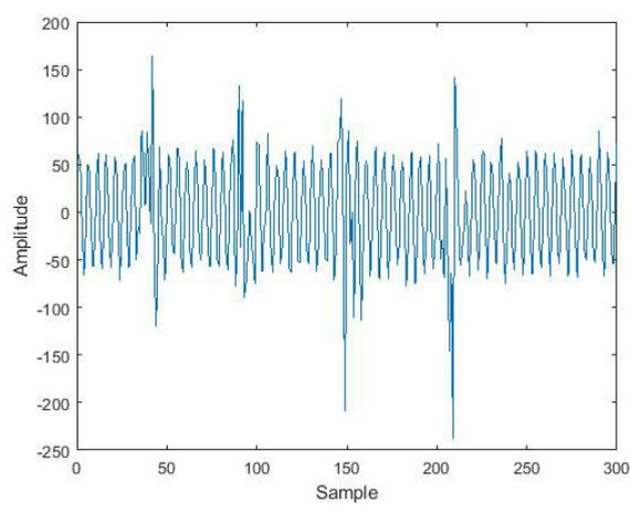
**FIGURE 11.** The DWT details coefficients of multiple eyeblinks (only ch1).
