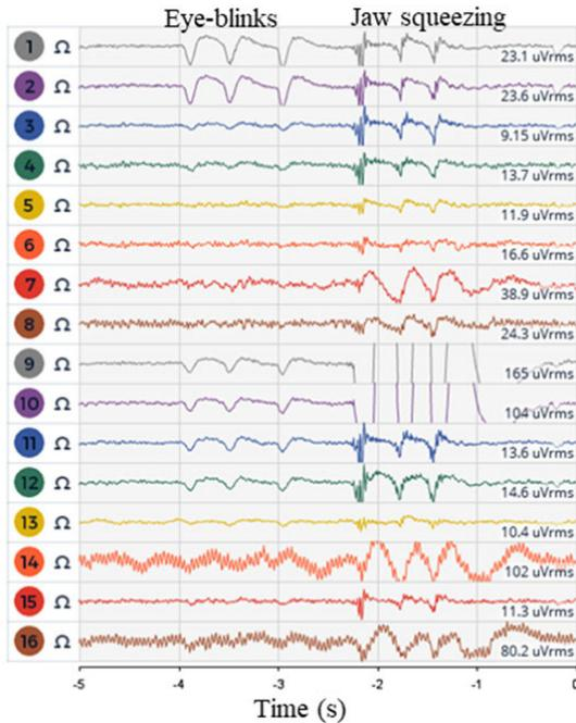
FIGURE 1. Eye-blink and jaw squeezing signals recorded by 16 channels using OPENBCI headset.
