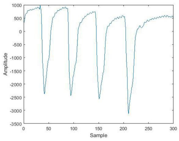
**FIGURE 14.** The DWT details coefficients of multiple jaw squeeze (only ch9).
