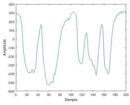
**FIGURE 10.** The DWT details coefficients of multiple jaw squeeze (only ch1).
