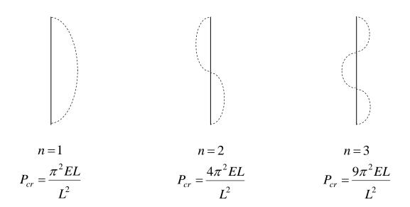
Critical buckling load: is the smallest value of axial load that can cause buckling.
