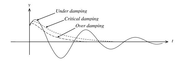
**Example:** A 10 kg mass is attached to a 1.5 m long spring. At equilibrium, the spring measures 2.481 m. If the mass is pushed up and released from rest at 0.2 m above the equilibrium position, find the displacement as a function of time, critical damping constant, natural frequency, and period of motion. (Assume the damping coefficient  $c = 20 \ N.s/m$ ).
