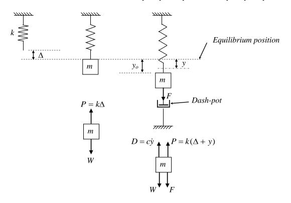
**Example 1:** A 5 kg mass is connected to a spring of 8.5 kN/m stiffness and subjected to an exciting dynamic force of 50cos30t kN. Assuming the viscous damping coefficient is 24% of the critical damping, determine the equation of motion of the mass. (Initial displacement and velocity are zero)
