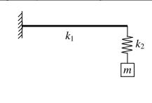
\* The equivalent stiffness for "in parallel" connection is,
