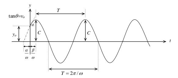
**Example:** A mass of 4 kg is attached to a spring of 1.6 kN/m stiffness. The mass is pulled down with a velocity of 0.6 m/s and released at 4 cm below the equilibrium position. Find the equation of motion, angular frequency, natural frequency, period of motion, and amplitude of motion (maximum displacement). Then, find the minimum time at which the mass passes through the equilibrium position.
