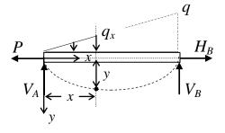
To determine  $M_x$ : From left;  $M_x = V_A x - Py - \frac{1}{2} q_x . x . \frac{x}{3}$ .  $\sum (M)_B = 0$ ,  $\frac{1}{2} qL \frac{L}{3} - V_A . L = 0 \Rightarrow V_A = \frac{qL}{6}$ .  $\frac{q}{L} = \frac{q_x}{x} \Rightarrow q_x = \frac{q.x}{L}$ .  $\therefore M_x = \frac{qL}{6} . x - Py - \frac{1}{2} . \frac{q.x}{L} . x . \frac{x}{3}$  $= \frac{qLx}{6} - Py - \frac{qx^3}{6L}$ .
