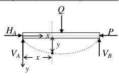
To determine  $M_x$ : From left;  $M_x = V_A.x + H_A.y$ .  $(0 \le x \le L/2)$   $\sum F_x = 0$ ,  $H_A - P = 0 \implies H_A = P$ .  $\sum (M)_B = 0$ ,  $Q \cdot \frac{L}{2} - V_A.L = 0 \implies V_A = \frac{Q}{2}$ .  $\therefore M_x = \frac{Q}{2}x + Py$ .
