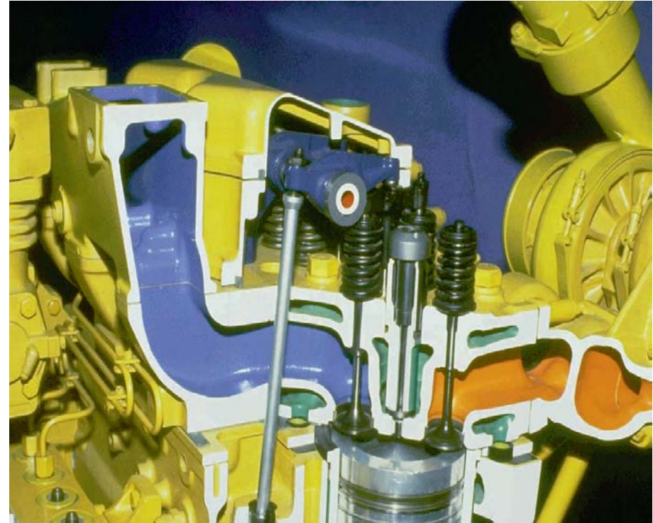
Each valve has a rotator which moves the valve face 3° relative to the valve seat during one complete cycle of the engine. This assures uniform wear for longer valve life and helps prevent burned valves.
