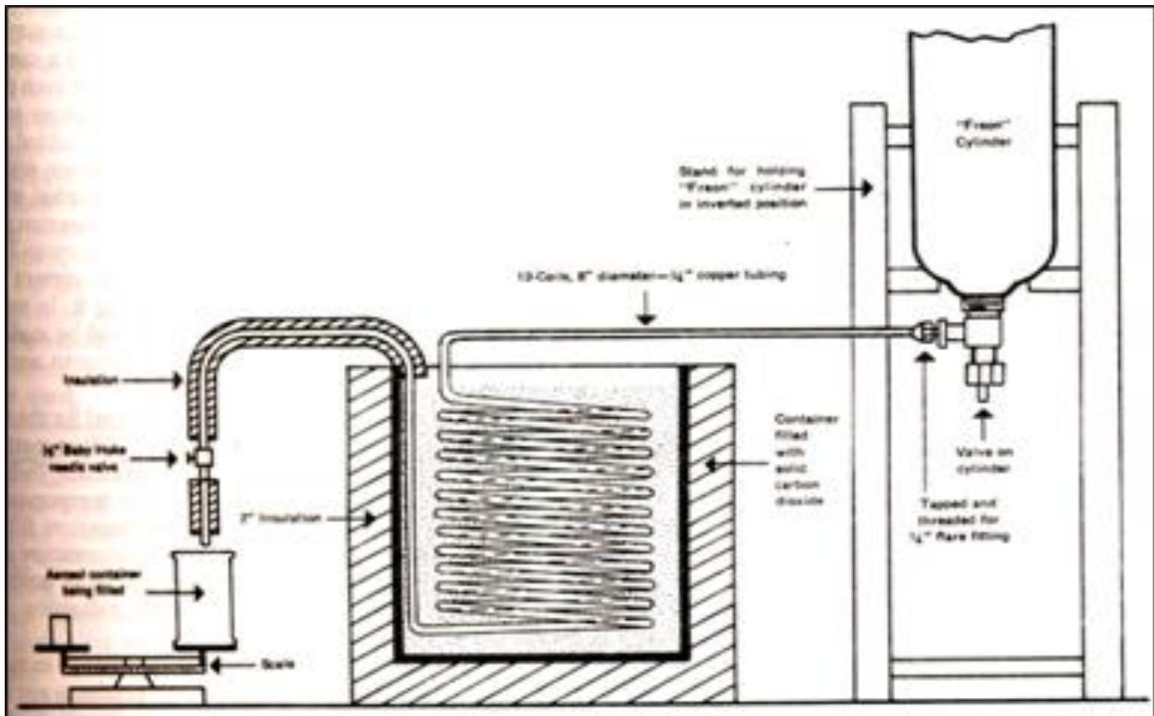
**Fig. 16. Aerosol Cold filling process Apparatus <sup>1</sup>**
