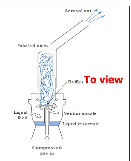
Fig. 37.10 • Schematic diagram of a jet nebulizer. Compressed gas passes through a Venturi nozzle, where an area of negative pressure is created. Liquid is drawn up a feed tube and is fragmented into droplets. Large droplets impact on baffles, and small droplets are carried away in the inhaled air stream.
