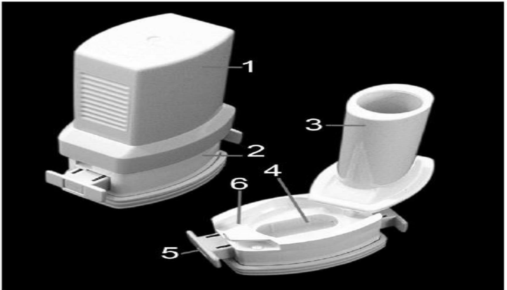
**Fig. 37.5 • The Aerolizer/Cyclohaler® dry powder inhaler. Comprising: 1 cap; 2 base; 3 mouthpiece; 4 capsule chamber; 5 button attached to pins for piercing capsule; 6 air inlet channel.**
