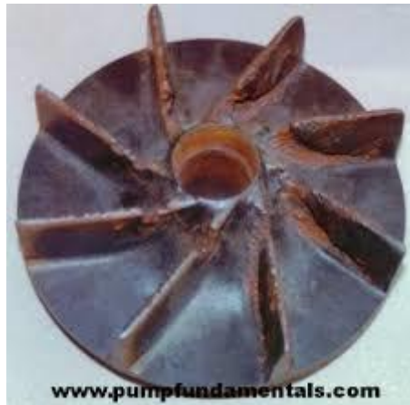
Fig.12 Cavities in pump impeller
