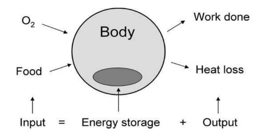
Change in stored energy in the body (i.e., food energy, body fat, body heat) → heat lost from body+Work Done • This is similar to the first law of thermodynamic:- $\Delta Q = \Delta u + \Delta w$
