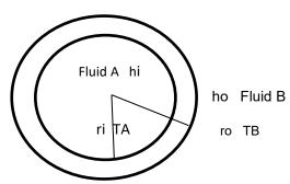
The area of convection is not the same, the terms Ai, Ao represent the inside and outside surface area of the tube .The overall heat transfer coefficient may be based on either inside or outside area of the tube.
