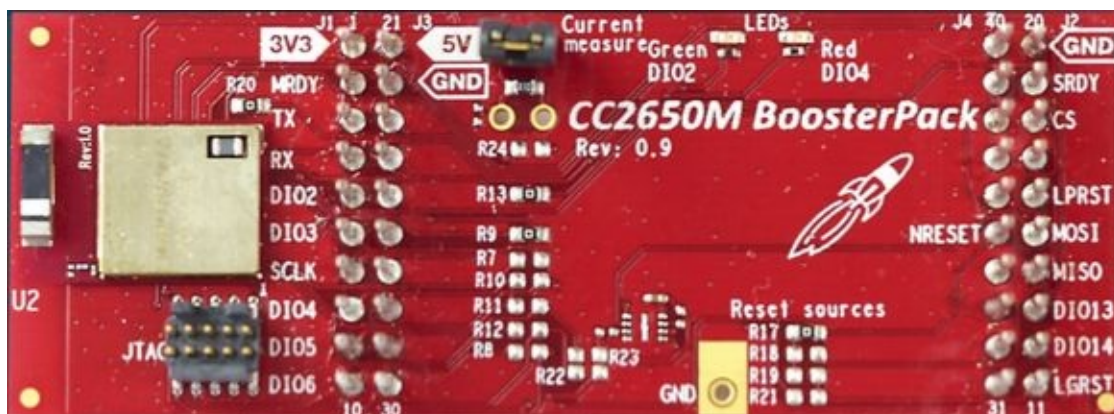
Figure 9.34. CC2650 BoosterPack (BOOSTXL-CC2650MA).
