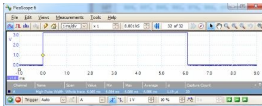
Figure 2.33. Oscilloscope output measured from Program 2.31 using a PicoScope 2104, running at 16 MHz.
