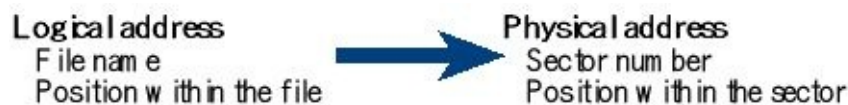
Figure 8.4. A file system must translate from a logical address to the physical address.
