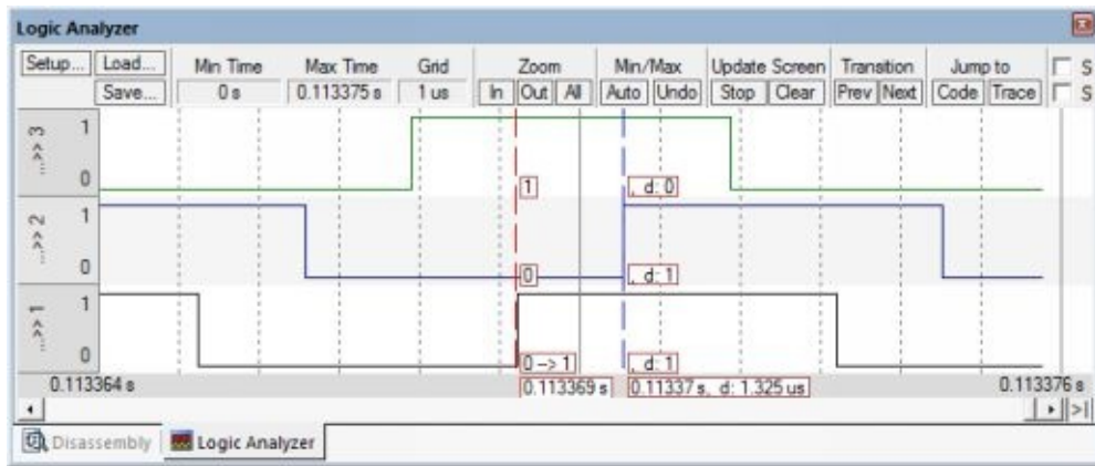
Figure 4.2. The OS runs three threads; each thread volunteers to suspend running in simulation mode on the TM4C123. The three profile pins from Program 4.2 are measured versus time using a logic analyzer.
