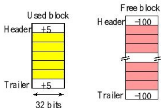
Figure 1.44. Each block has a header and a trailer.
