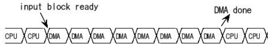
Figure 7.6. An input block is transferred all at once during burst mode DMA.
