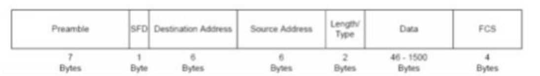
Figure 9.22. An Ethernet frame can hold 46 to 1500 bytes.
